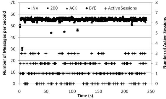
Fig. 19. RE message processing rates with ICS+MB+SF
