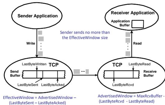
Fig. 4. TCP flow control
