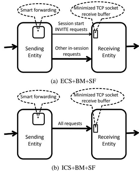
Fig. 30. SIP-over-TCP overload control mechanisms after parameter simplification
