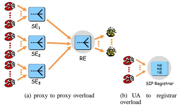
Fig. 3. Types of SIP server overload
