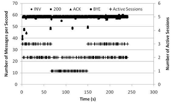
Fig. 13. RE message processing rates with ECS+MB+SF
