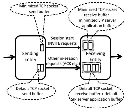
Fig. 10. Explicit Connection Split + Buffer Minimization
