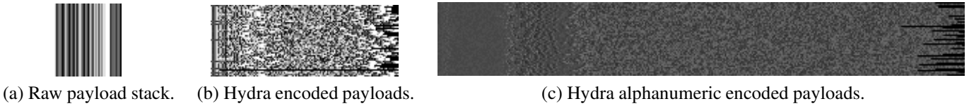
Figure 20: Spectral images. Each row represents a shellcode sample, the intensity of the pixels are given by the byte values of each instance (row) and the color spectrum is normalized to [0,255] . Basic encodings are shown: no NOP-sled, 5-layer cipher, no spectrum blending, no return address zone. Alphanumeric encodings map to a smaller (and darker) color spectrum, as shown in (c). The lengths of the encoded shellcode also vary.
