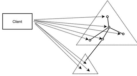
**Figure 3. The pair-wise key distribution across SOA boundaries used in the naive public-key implementation. The client must store a key for each destination node in the SOA and each node of its children SOAs.**
