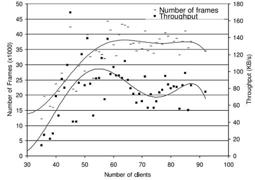
Fig. 4. Throughput and num. of frames vs. num. of clients on channel 6
