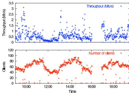
Fig. 3. Total throughput and number of clients on channel 6
