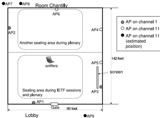
Fig. 1. Measurement and network setup in Chantilly
