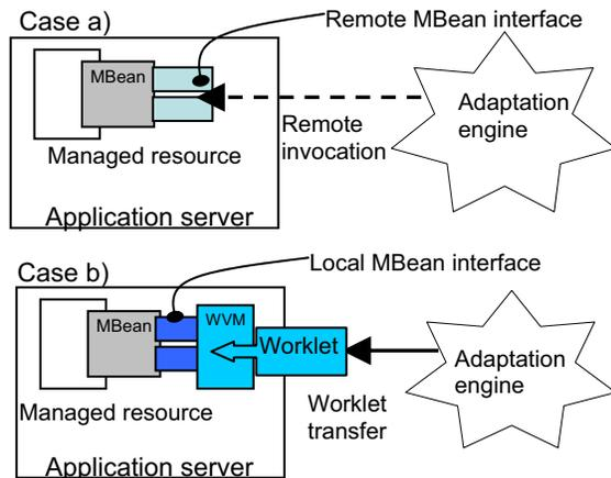
**Figure 4: Interfacing JMX adaptation provisions to Worklets.**
