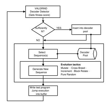
Figure 1: *Decoder search engine flow chart*. An overview of our decoder search engine. We construct our library of decoders using a feedback loop that creates candidate decoders, confirms that they exhibit sufficient decoding behavior, and uses them to generate more samples.
