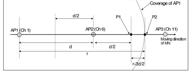
Fig. 1. AP arrangement where false handoff can occur with passive scanning
