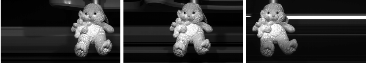
Figure 10: Pushbroom panoramas of a moving object produced by the system in Fig. 8. The size of each image is 4000 \times 1024 [pixel] (the images were cropped for display purposes). The left and middle panoramas were used to recover velocity, while the middle and right panoramas were used to recover 3D structure.
