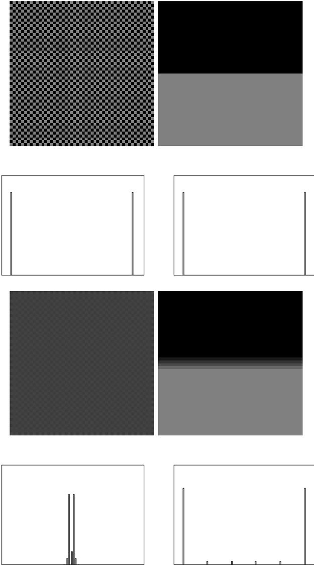
Fig. 3. An example illustrating the usefulness of multiresolution histograms. The top row shows 2 very different scenes at full resolution, with their corresponding histograms in the second row. The third row shows these scenes blurred to  $1/2$  resolution, with their corresponding histograms in the last row.
