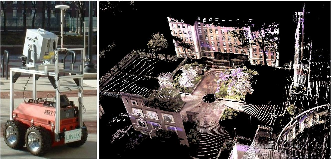
Fig. 1. The ATRV-2 Based AVENUE Mobile Robot (left). A sample laser scan taken with the AVENUE system on the Columbia University campus (right). The hole at the center of the scan is where the scanner was positioned.
