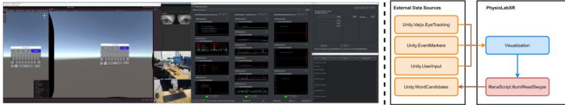
Figure 14: SwEYEpe enables a Swype-like process using eye tracking in virtual reality. The system inherits all the typing keyboard functions of the iOS system, and users can trigger SwEYEpe with a button press. The image above demonstrates that the user was typing “Virtual Reality,” and the spelling correction algorithm carried out the correct suggestion.
