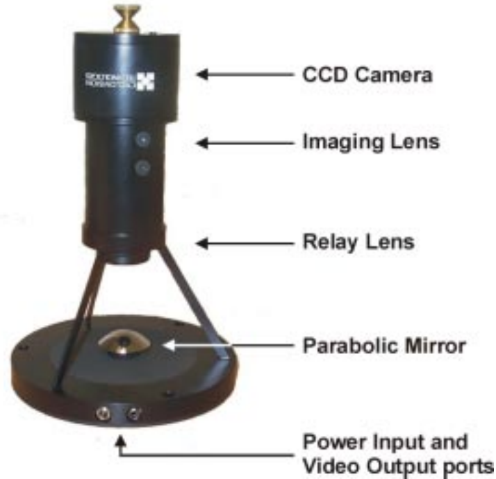
Figure 6: The omnidirectional camera that is mounted on top of the PARAROVER chassis.
