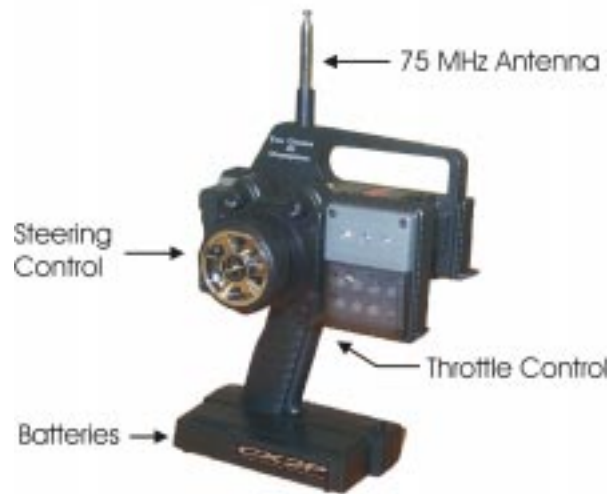
Figure 5: The hand-held radio controller that allows the user to cause the PARAROVER to accelerated, decelerate and turn.
