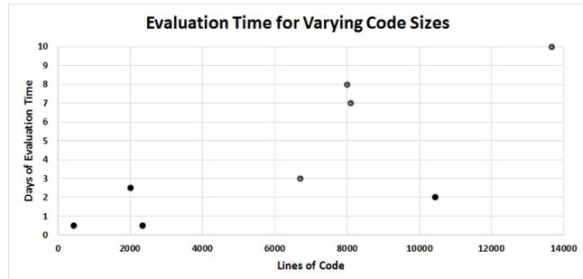
**Figure 2: Trade-off between lines of code analyzed and runtime. The black points denote designs that finished completely in the contest time frame. The lighter points represent designs that were analyzed partially for the contest. For those points, the full runtime is estimated.**
