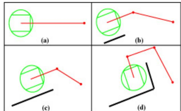
**Figure 2.** (a) Initial path to goal. (b) Side sonar detects an obstacle; a new path is generated in order to avoid frontal collision. (c) Side obstacle is still detected, a new segment is added to its representation. (d) A frontal obstacle is now detected, waypoints are added in order to avoid it
