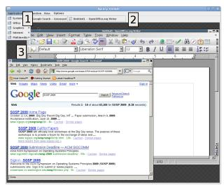
Figure 1: Apiary screenshot showing a user's desktop session. At the the topmost left, (1) An application menu that provides access to all the applications available to the desktop. Just below it, the window list (2) allows users to easily switch among running applications and the composited display view (3) of all the visible running applications.
