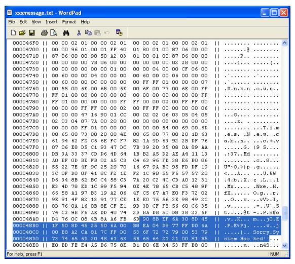
Figure 4: The binary content of a malicious shellcode embedded in a Word document (fcSttbfffn).
