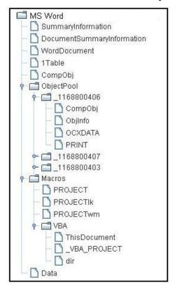
Figure 2: An example of the internal structure of a parsed document in OLE format
