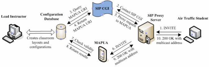
Figure 4. Call flow diagram for radio line communication
