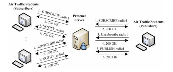
Figure 7. Call flow diagram for notification of transmissions
