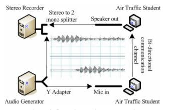
Figure 8. Setup for audio latency testing
