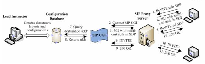
Figure 5. Call flow diagram for land line communication
