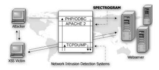
Fig. 2. Spectrogram is a web-layer, network situated sensor.
