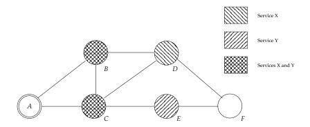
Figure 1: The desired scope of services announced from host *A*.
