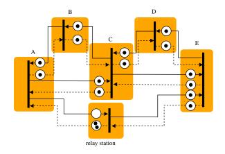
Fig. 15. An LIS where relay-station insertion is not enough.
