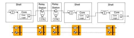
Fig. 4. Marked-graph model (with q = 2) of a path across multiple shells and relay stations in a LIS.
