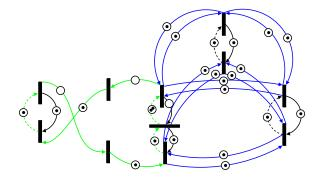
Fig. 20. Adding a Relay Station to the Edge construct.
