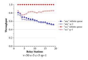
Fig. 16. MST of graph (v=50,s=5,c=5,rp=1) given infinite and finite (q=1) queues.
