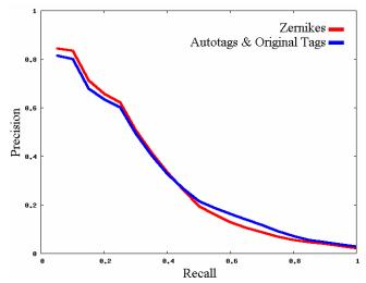
Fig. 4. The precision/recall for our autotags combined with the original tags is very similar to the precision/recall of the Zernike descriptors.
