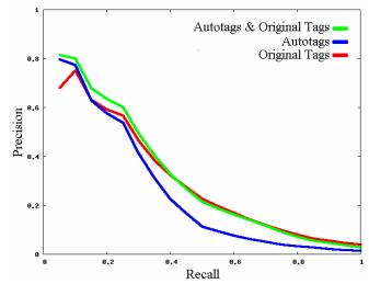
Fig. 3. The precision/recall for the original tags combined with our autotags is better than either set of tags individually.
