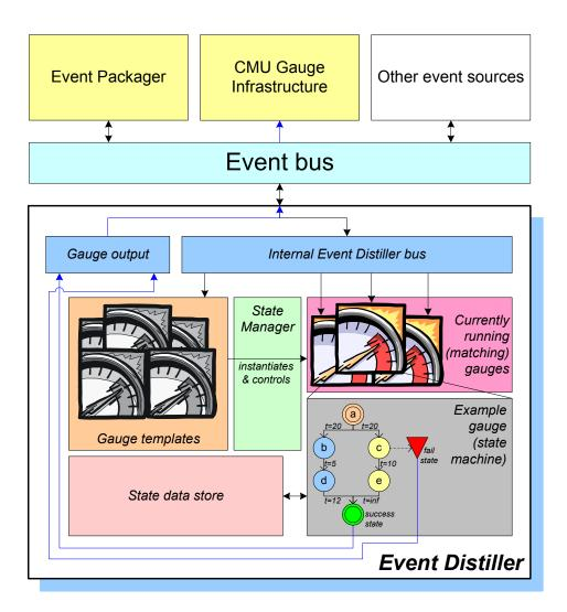
Figure 2.3: Event Distiller Internal Architecture.
