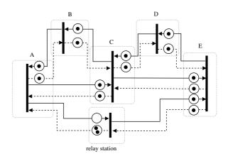
Figure 7: An LIS where relay-station insertion is not enough.
