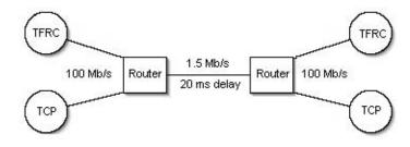
Fig. 2. Dumbbell Topology for experiment simulation.
