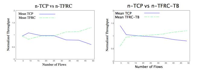
Fig. 3. Normalized mean throughput of TCP flows competing with TFRC or TFRC-TB flows over shared bottleneck link.
