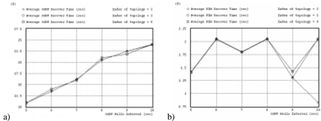
Fig. 8. a) Variation of OSPF topology updating time with the OSPF Hello interval. b) The time between topology updating by OSPF and multicast channel recovery using PIM, as a function of the OSPF Hello interval
