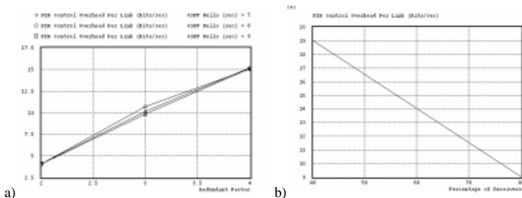
Fig. 6. PIM DM load change with the variation of network redundancy factor a) and receiver percentage b)
