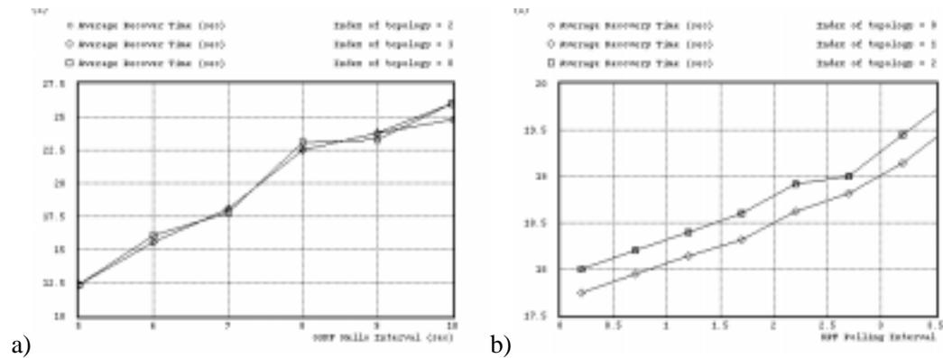
Fig. 7. a) Variation of multicast channel recovery time with the OSPF Hello interval (PIM polling interval set to 0.2 s) b) Variation of multicast channel recovery time with the PIM polling interval
