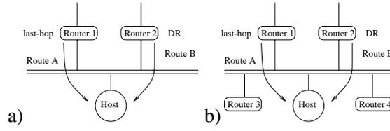
Fig. 2. LAN failure scenario, DR and last-hop router are different routers
