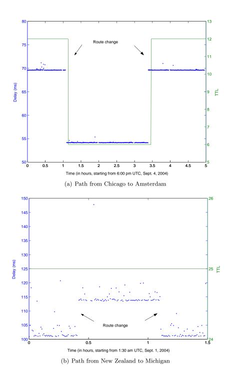
Figure 10: Delay variation and TTL based route change detection
