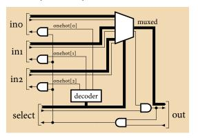
A multiplexer takes a *select* input and uses it to steer the data and *valid* signals from the selected input to the output when *select* is also valid. If the downstream is ready, the token on *select* and the corresponding input is consumed.
