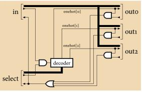
A demultiplexer is mostly handshaking. The data fans out, but at most one output is valid when the input and *select* channels have data. When they do, *select* sets which output is valid, and the input and *select* tokens are consumed only when the selected output is also ready.
