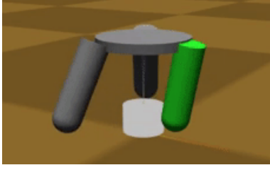
Fig. 6. Gripper fingers bounced off of the block even though the Coefficient of Restitution = 0, the applied forces are all equal, and the fingers are oriented the same way.
