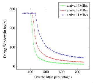
**Figure 6.** Simulation results for debug-window size. Each series has a constant arrival rate, and the buffer is kept at 64GB.
