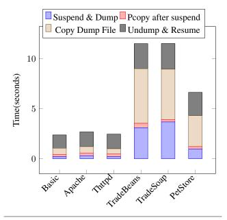
**Figure 4.** Suspend time for live cloning, when running a representative benchmark
