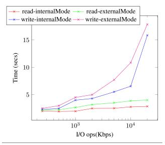
Figure 5. Live Cloning suspend time with increasing amounts of I/O operations
