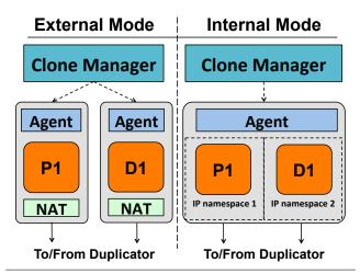
**Figure 3.** External and Internal Mode for live cloning: P1 is the production, and D1 is the debug container, the clone manager interacts with an agent which has drivers to implement live cloning.
