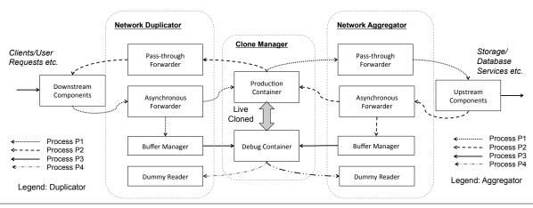
**Figure 2. High level architecture of** *Kensa*, showing the main components: Network Duplicator, Network Aggregator, and Cloning Manager. The replica (debug container) is kept in sync with the master (production container) through network-level record and replay. In our evaluation, we found that this light-weight procedure was sufficient to reproduce many real bugs.
