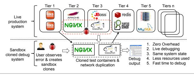
**Figure 1.** Workflow of *Kensa* in a live multi-tier production system with several interacting services. When the administrator of the system observes errors in two of it's tiers, he can create a sandboxed clone of these tiers and observe/debug them in a sandbox environment without impacting the production system.
