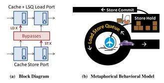
**Figure 1. Store Forwarding Mechanism.** The subcomponent hardware is represented by a block diagram in (a) and a traffic metaphor in (b). The metaphor provides an intuitive visualization of the component behavior.
