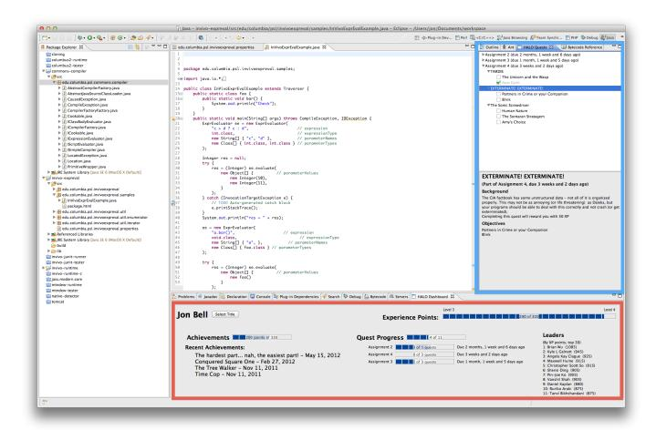
Fig. 1: The HALO Eclipse plugin: The bottom part (highlighted in red) shows the dashboard, which keeps track of the achievements, experience points, leaderboards; The top right part (highlighted in blue) shows the quest list and progress
