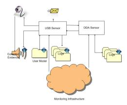
Fig. 1. Architecture of the RUU Masquerade Attack Sensor
